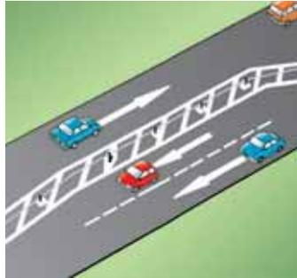
There may be a safety barrier in the centre of the road which separates the two directions of traffic and prevents drivers from overtaking in the one-lane section. If vehicles need to turn right, they can do so at junctions.
