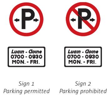
The sign below shows a clearway – an area of road that **must** be kept clear for moving traffic during certain times of the day (usually busy periods). The times when stopping or parking is prohibited are shown on an information plate under the sign.
